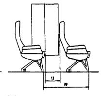
Configuration (M) SEAT PITCH - 39 INCHES VERTICAL PROJECTION - 13 INCHES EQUIVALENT TO AN 79 REQUIREMENTS
